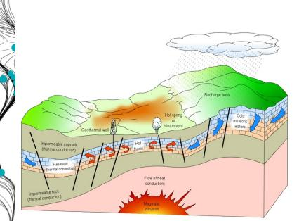
Conceptual geothermal system with steam extraction for electricity production and surface manifestations source: Geothermal-energy.org
